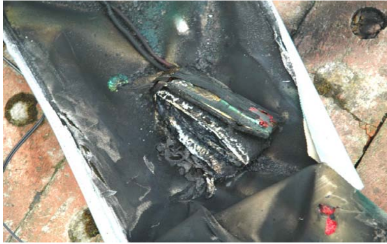
The remains of a burnt-out LiPo still in a safety sack.
